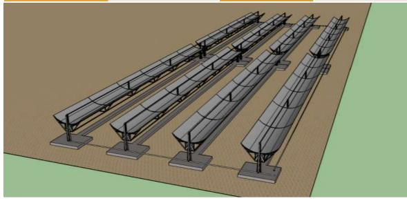
Table 3: Proposed parabolic through collectors solution. Initial demand.
